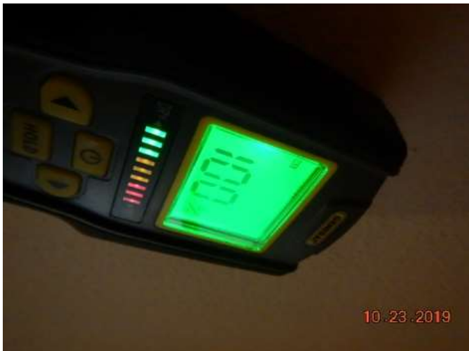
High moisture reading
