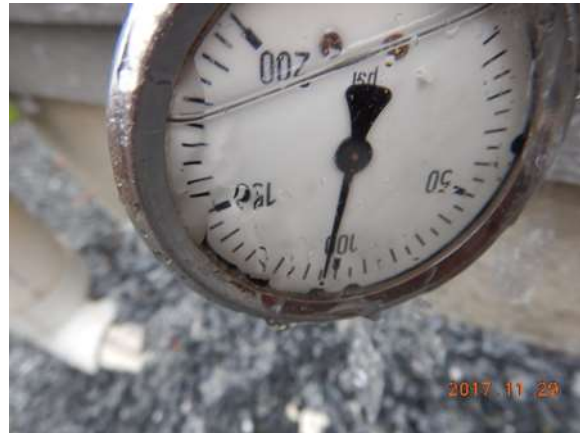
Water pressure is excessive (> 80 PSI)
