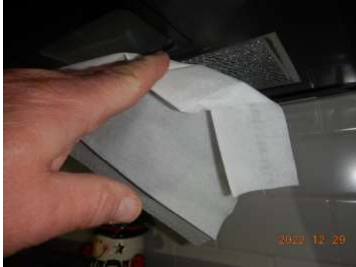
The ventilation system cannot lift a tissue when set to the “high” position
